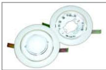
Recessed mounting base is used for mounting conventional as well as analogue addressable detectors on false ceilings of various types (metal, plaster etc.). The base allows creating more aesthetic architectural applications. Bases are produced from ABS and have the same colour as detectors. Bases are flush-mounted into ceiling with two clamps and stainless steel screws.
